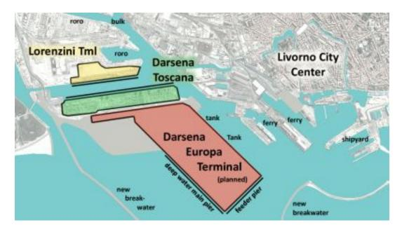
The port of Livorno (aka Leghorn) has recently carried out dredging to improve vessel access to its container terminals. Livorno's aim was to facilitate calls from 10,000 teu class container vessels with a draft of up to 12.00 m compared to just 10.75 m in the past.
